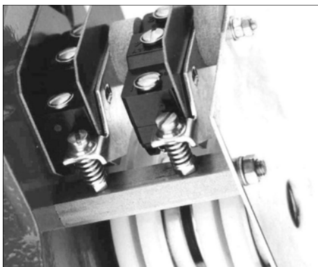
Fine adjustment by matching screws
