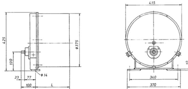
Construction II for max. 16 contacts. Optional position of installation
