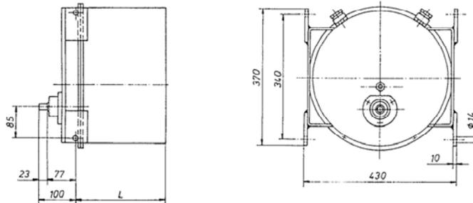
Construction III for max. 24 contacts. Horizontal position of installation
