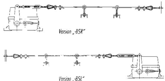
switch by lifting the blue lever. Upon releasing the pullcord must be shortened in that way, that the actuation lever stands upright (like in the sketch right beside). This is the neutral position of the switch. Check: Pulling on the rope should effect actuation and latching of the switch. Release by the blue lever.
