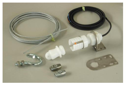
In order to be able to detect damage to the conveyor belt as best as possible, a rope is attached transversely and as close as possible to the conveyor belt. One end of this rope is fixed to the structure of the conveyor. On the other side it is connected to a male plug socket which is held in a female plug socket.
